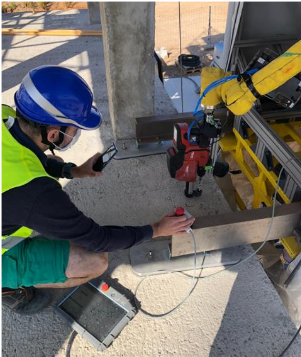
Figure 13. Co-author K. Iturralde checking the performance of the modular end-effector of the HEPHAESTUS robot (photo: S. Palencia Ludeña)
