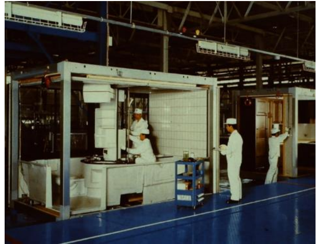
Figure 1. Stationary construction robotics of the Misawa-Toyota Homes assembly line (photo: T. Bock)
